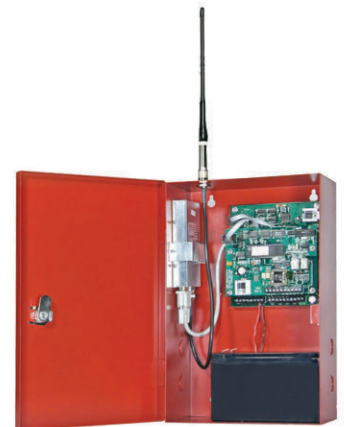
Even if an intruder cuts the exterior phone line, an alarm with radio backup installed will continue to function.
